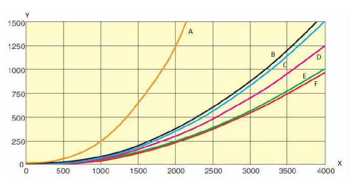
Y= Pressure drop (Pa), X= air flow (m3/h) A = Trolley fume extractor arm B = Top Outlet - side  $\emptyset$ 250 C = Maxi Trolley  $\emptyset$ 200 without hose D = Rail end outlet ALU 250 /  $\emptyset$ 250 E = Top outlet  $\emptyset$ 250 F = Rail end outlet ALU 150 /  $\emptyset$ 250
