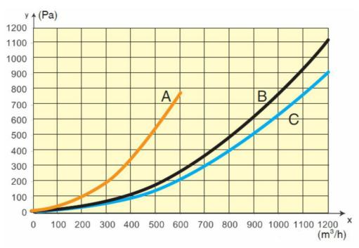
Pressure drop extraction units with A= hose Ø 100 mm, 5 m B= hose Ø 150 mm, 7.5 m C= hose Ø 150 mm, 5 m
